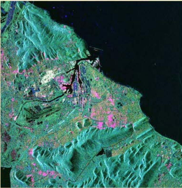
Fig. 2. This polarimetric decomposition-based RGB image of EOS-04 over Visakhapatnam, India, highlights distinct scattering phenomena: red represents double-bounce scattering, blue indicates single-bounce scattering, and green denotes volume scattering elements
